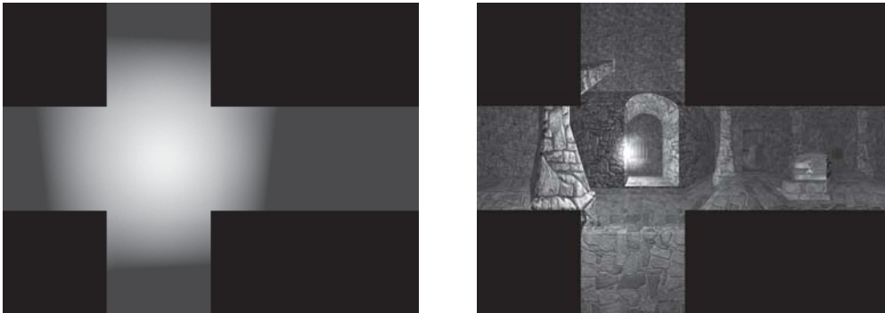
Figure 1: Diffuse cube map (right) and reflection cube map (left) for one light
