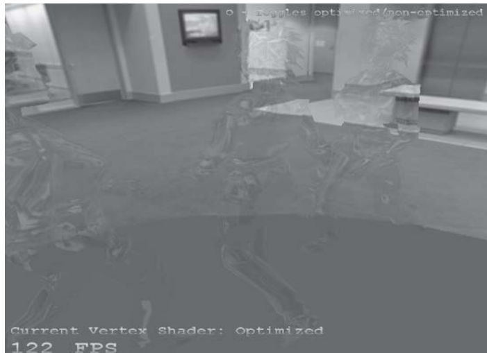
Figure 5: Skinned mesh soap bubble shader example. Vertex shader is performing skinning, sinusoidal perturbation, reflection, and refraction calculations for texture coordinates.
