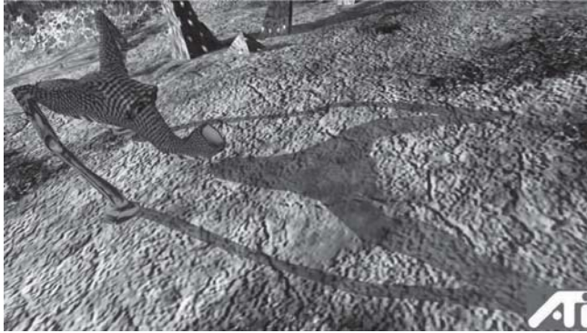
Figure 4: Artifacts caused by skinned face normals. Notice the notch in the shadow of the shoulder.
